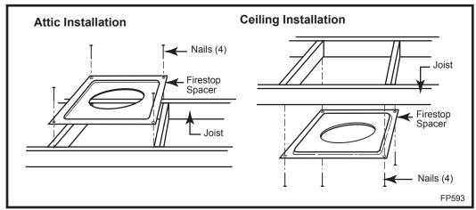
Fig. 18 Installing firestop spacer.
